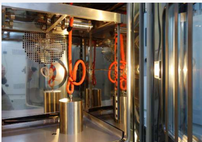
Cold Bend Cables Testing
