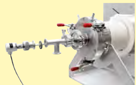
Thermocouple for charge control
