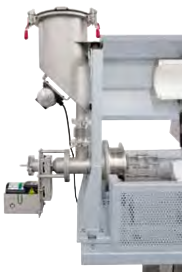
Vibration unit at the charging funnel for improved powder supply
