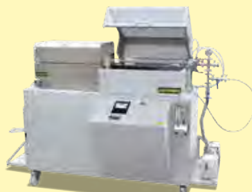
RSH 120/500/11S with sliding furnace
