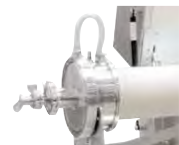
Water-cooled vacuum flange (gas supply system 2)
