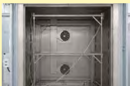
Pluggable frame for measurement for forced convection chamber furnace N 7920/45 HAS
