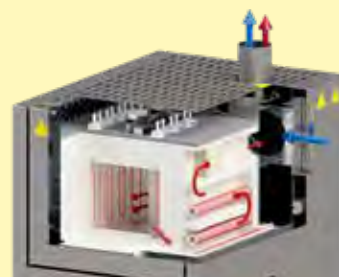
Schematic representation of the air flow in combi furnace LHT 08/17 BO
