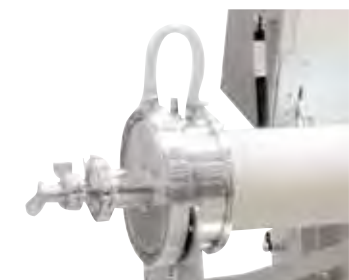
Water-cooled vacuum flange (gas supply system 2)
