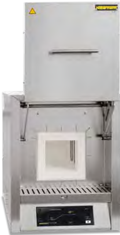
High-temperature furnace LHT 02/17
