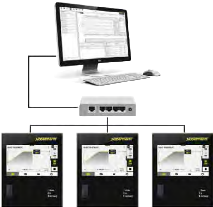
Example lay-out with 3 furnaces
