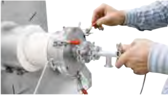
Water-cooled stainless steel flanges with quick locks as additional equipment
