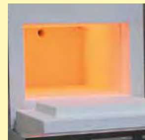
Muffle heated from four sides
