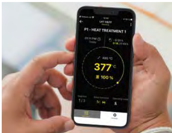
Display of program progress for each furnace
