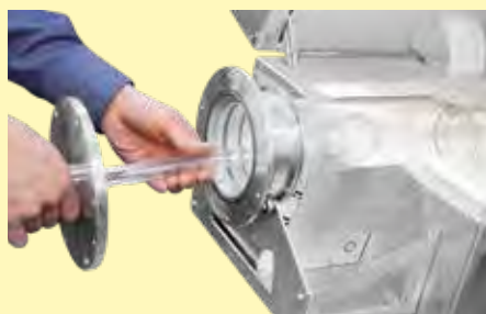
Gas tight closing plug for tubes made of quartz glass closed at one side as additional equipment
