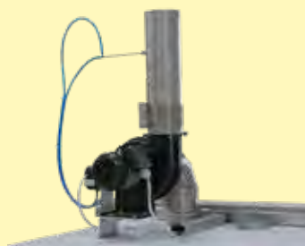
Fresh-air opening and powerful exhaust air fan installed on the furnace
